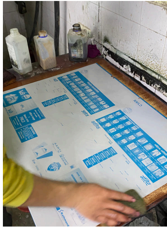
Preparing: Cleaning the plate with alcohol and plate cleaning chemical
