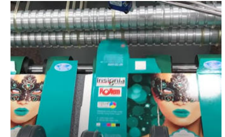
4. Packaging is cut according to the dielines
