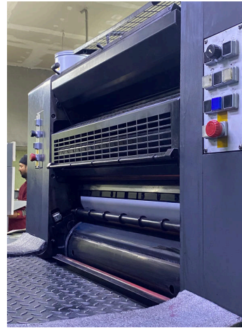
Each segment is for a different color: Generally, 4 compartments for CMYK
