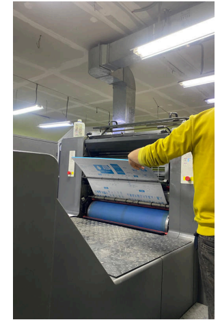
Plates are fed according to colors. Eg: A yellow plate is being entered
