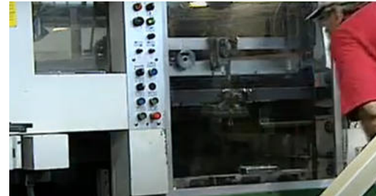
3. Die-cutting machine firmly presses the die into the material to cut out the shape
