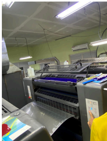
Cyan plate loads on roller. Ink applied. Only one plate at a time.
