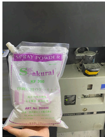
Near the end, spray powder is added inside the machine to prevent ink smudging and papers sticking together.
