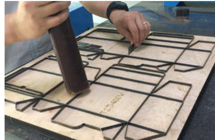
2. Steel rules are hammered into the die board
